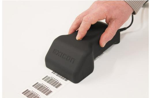
The 6500 series can be operated either horizontally or vertically (on the side of a carton) but always in contact with the barcode. The 6500 series verifier cannot be used for symbols wider than 125mm, and this dimension includes the quiet zones.
